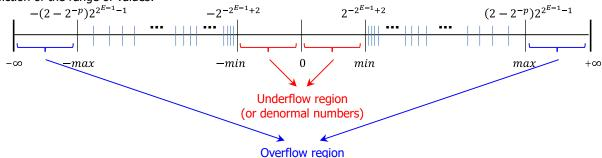
■ The IEEE-754-2008 (revision of IEEE-754-1985) standard defines several representations: half (16 bits, E=5, p=10), single (32 bits, E = 8, p = 23) and double (64 bits, E = 11, p = 52). There is also quadruple precision (128 bits) and octuple precision (256 bits). You can define your own representation by selecting a particular number of bits for the exponent and significand. The table lists various parameters for half, single and double FP arithmetic (ordinary numbers):
