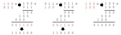
**Note**: If one input is negative and the other is positive, we can use the negative number as the multiplicand and the positive number as the multiplier. Then, we can operate as if it were unsigned multiplication, with the caveat that we need to sign extend each partial sum to 2n bits (if both operators are n-bits wide), or to n + m (if one operator is n-bits wide and the other is m-bits wide).
