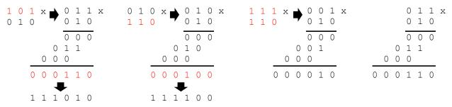
■ **Note**: If one of the inputs is  $-2^{n-1}$ , then when we change the sign we get  $2^{n-1}$ , which requires n+1 bits. Here, we are allowed to use only n bits; in other words, we do not have to change its sign. This will not affect the final result since if we were to use n+1 bits for  $2^{n-1}$ , the MSB=0, which implies that the last row is full of zeros.
