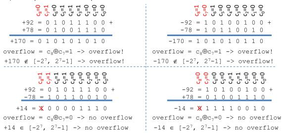
• To avoid overflow, a common technique is to sign-extend the two summands. For example, for two 4-bits summands, we add an extra bit; thereby using 5 bits to represent the operators.
