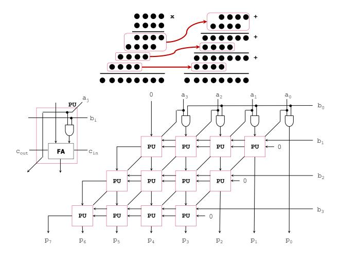
11 Instructor: Daniel Llamocca  An alternative array multiplier is depicted in the figure below: at every diagonal of the circuit, we add up all terms in a column of the multiplication. Every stage (row) does not propagate the carries to the left; instead, they are sent down to the next stage. Only the last stage propagates carries to the left.
